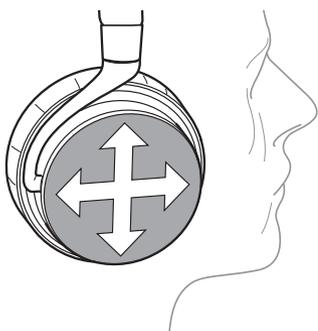
The Touch controls are located over the whole outside surface of the right ear shell.
